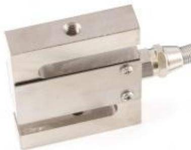
An S-type load cell. By pulling on both ends or pushing on both ends, the stress in the S changes and the cell's output changes.
